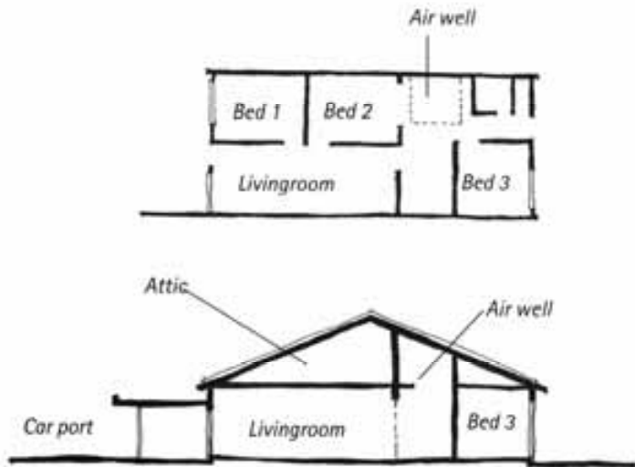
10.17 Plan and section of an air well showing thermal dynamic forces
