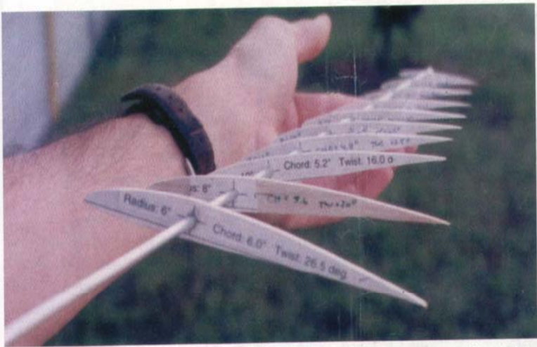
Partway through construction, prototype blade maker Jeff Sonne holds the first of four airfoils he would build by hand. He cut balsa sections of the airfoil from the computer-generated plot.
