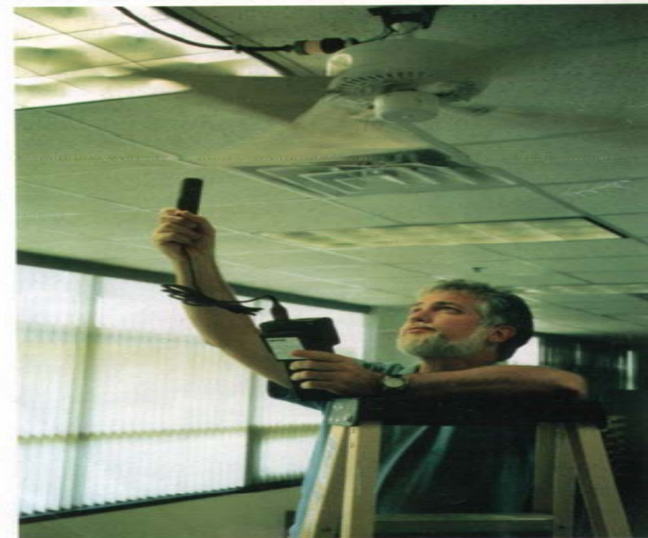
Using an infrared tachometer, Parker checks prototype's speed during efficiency testing. Fans were evaluated for airflow and power consumption, too.
