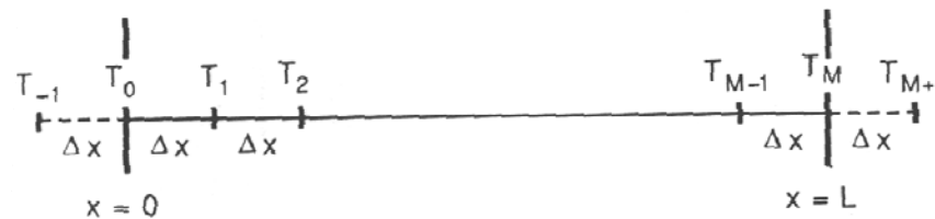
Figure 3-2 Fictitious nodes at fictitious temperatures T_{-1} and T_{M+1} .
